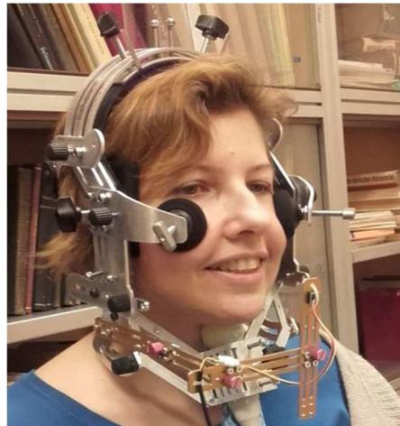
**Figure 1:** Ultrasound stabilization helmet with the fixed ultrasound transducer and lip camera (in the front of the lips)
